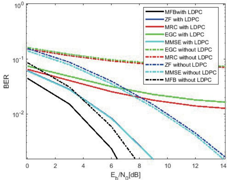
Figure 2. Results for RS System, with 3 users and 50 antennas, with /without LDPC codes.
