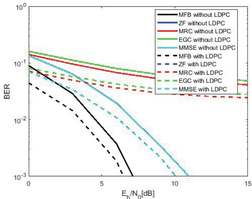
Figure 4. Results for RS System, with 12 users and 200 antennas, with/without LDPC codes.
