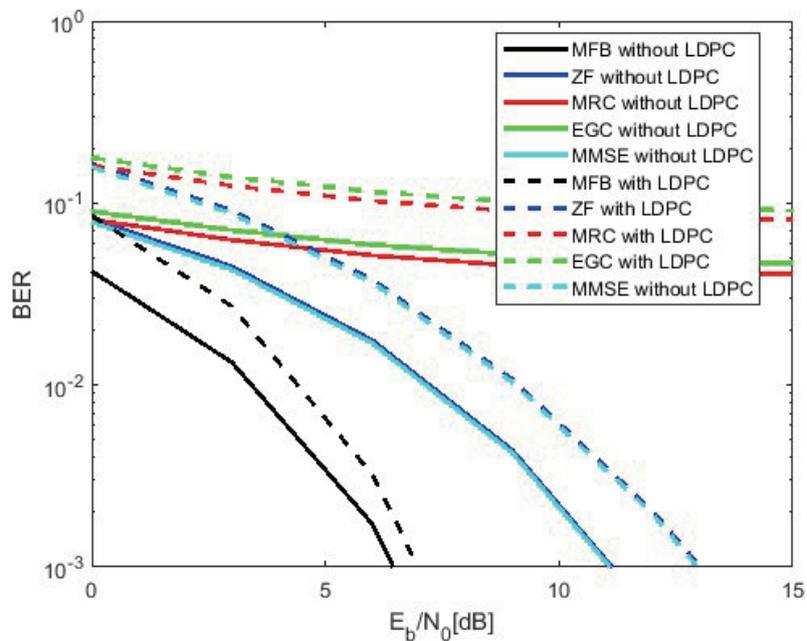
Figure 3. Results for RS System, with 6 users and 100 antennas, with/without LDPC codes.
