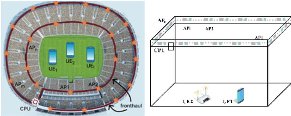
Figure 1. A radio stripe installed along the stadium and walls [2].
